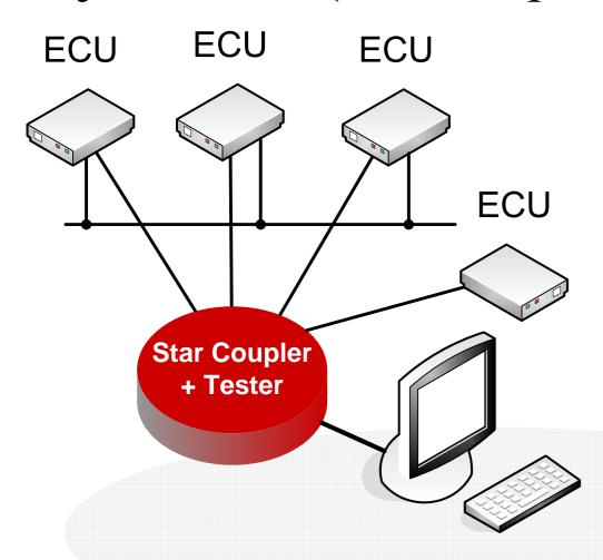
The approach in the DECS project is to integrate the tester – consisting of (i) bus monitoring, (ii) replay and (iii) fault injection functionality – with a star coupler. The embedded tester node is controlled by a host PC that uses a highspeed USB2.0 interface for control & data transfer.
