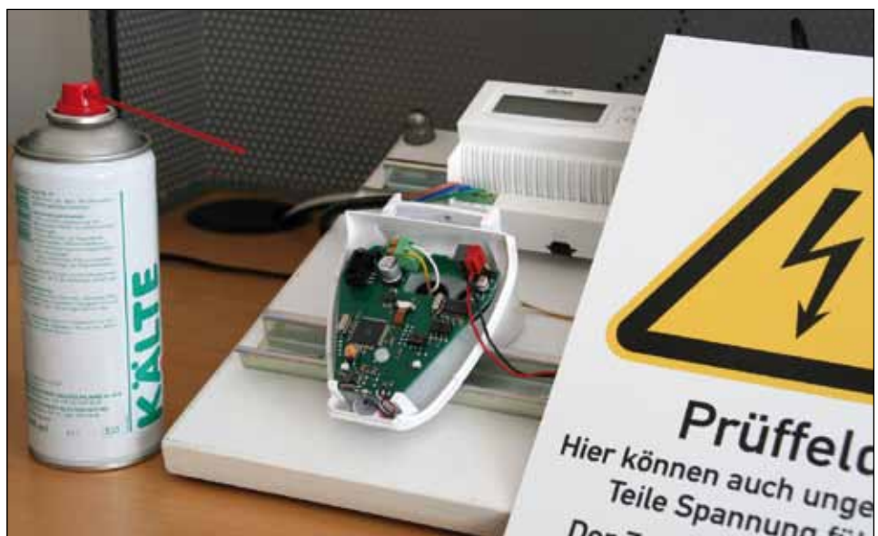
Test setup for a weather sensor. The wind sensor can easily be influenced with ice spray.
