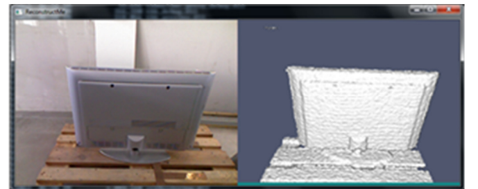
Figure 6: Reference scan of the TV-set with ReconstructMe
