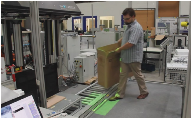
Figure 4: The assistance system is providing instructions and light patterns (green light on the shop floor) to guide the worker.
