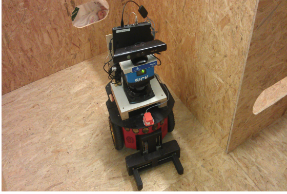
Fig. 4. Pioneer DX-3 robot with SICK laser sensor for mapping.
