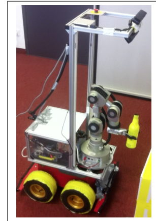
Fig. 1. The Robot P3AAT at the attempt to grasp the bootle.
