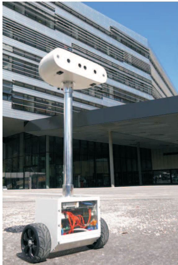
Fig. 1. The two-wheeled, self-balancing mobile robot in front of the newly built Science Park of the Johannes Kepler University Linz
