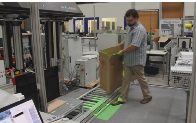
Figure 4: The assistance system is providing instructions and light patterns (green light on the shop floor) to guide the worker.
